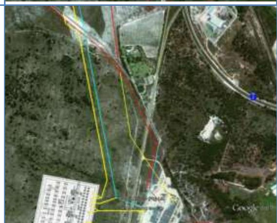
(ix) Provisioned to reroute the Hermanus 66kV feeder to the MTS when increased to 132kV in the future.
