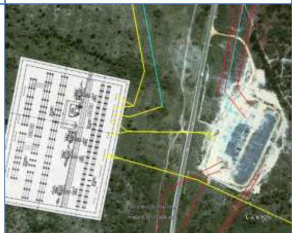
(viii) Provisioned to allow double circuit 132kV to the northern wind farm from the existing Houhoek S/S by moving Lebanon Switching 1 over to the old Lebanon 2 structure (would require re-conductoring and rebuilding of a section of the Lebanon Switching 2 line, with a single circuit up to a point and a D/C 66kV to connect the Houhoek-Vyeboom 66kV line by diverting it to the 66kV busbar at the back of the substation using two 66kV feeder bays. This would avoid crossing the 132kV feeder bay.
